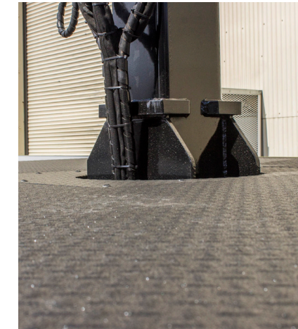
Base plate is installed flush to truck bed for safer operator use.
