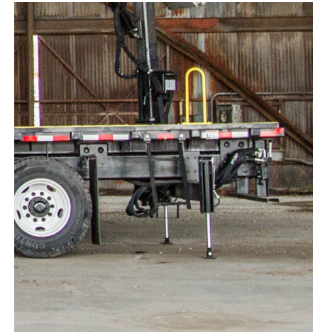
Vertical lift reduces chance of surface damage.
